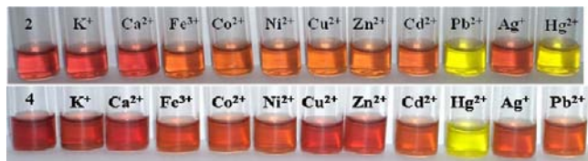
Figure 3. Changes in the color of solutions of 2 ( c = 100 \mu\text{M} ; \text{H}_2\text{O}:\text{EtOH} , 50:50, v/v; \text{pH} \approx 7.2 ) and 4 ( c = 100 \mu\text{M} ; \text{H}_2\text{O}:\text{MeCN} , 10:90, v/v; \text{pH} \approx 7.6 ) with 10.0 equiv of various metal ions (100 mM).
